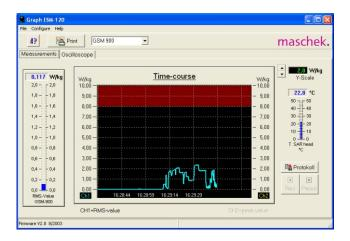
With the fibre optic cable delivered along with the meter, the ESM-120 can be operated free of interferences and independent of the mains. It is also possible for it to be integrated in automatic test benches.
